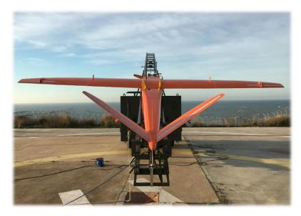
The **MOAI** can be used as a direct target, but because of its powerful motor, it can also tow a wide range of sub-targets depending on the type of mission. This aerial target can be fitted with several payload, such as the MDI (Miss Distance Indicator), which report in real time the distance at which the bursts fired by the defence system operator pass from the target, radar or infra-red signature enhancers, smoke cans, etc.
